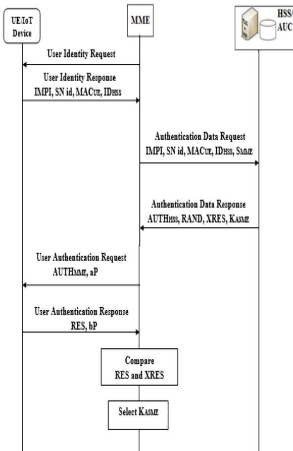
Figure.6 Proposed LTE authentication procedure
