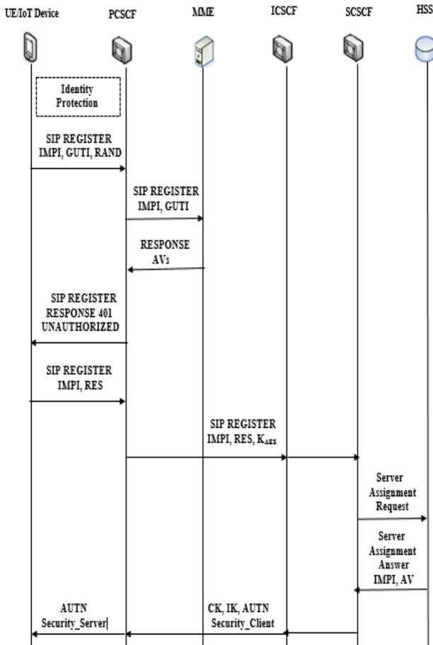
Figure.7 Proposed IMS authentication procedure
