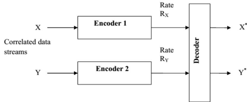
Figure.2 independent encoding and joint decoding of two correlated data streams X and Y
