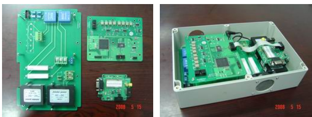
Figure 5 Implementation of the sensing, processing and transmitting unit (WSN node)
