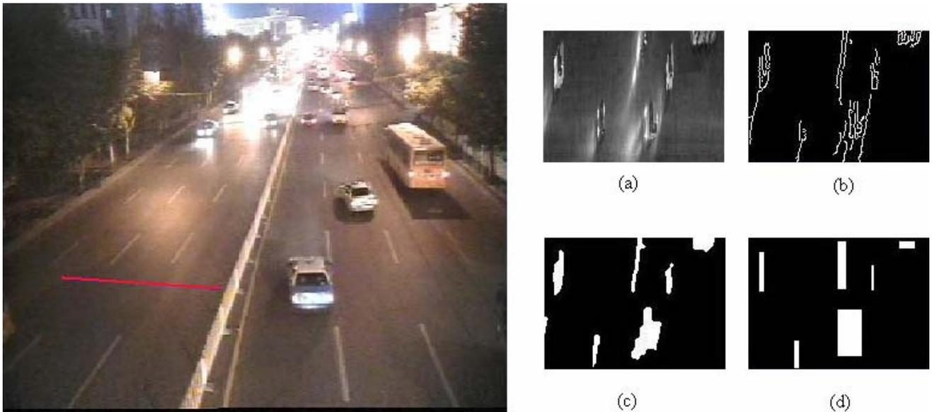
Figure4. A video frame of night situation with headlight impact (left). The length of virtual detection line is 110 pixels. (a) Time-spatial image in headlight impact situation. (b) Image after edge detection. (c) Image after morphological close operation and hole filling. (d) Image after moment computing
