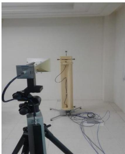
Figure. 22 Photograph of the proposed antenna during the measure of the gain
