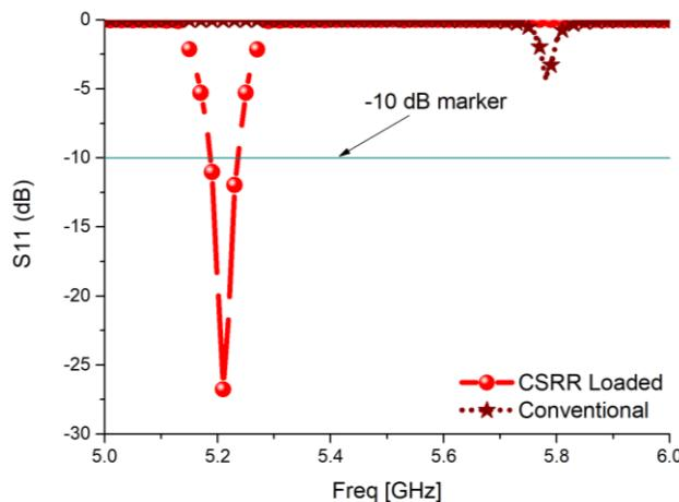
Figure. 3 Simulated S11 of the conventional and CSRR loaded antennas
