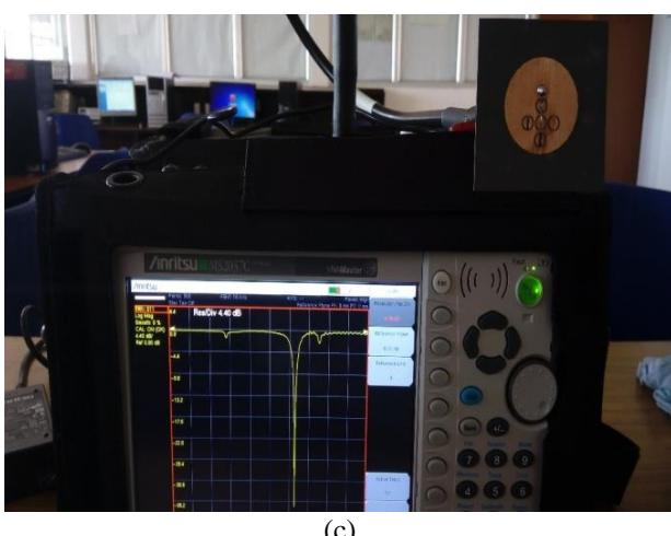
Figure. 6 Prototype and measurement setup: (a) top view of the prototype, (b) bottom view of the prototype, and (c) S11 measurement setup
