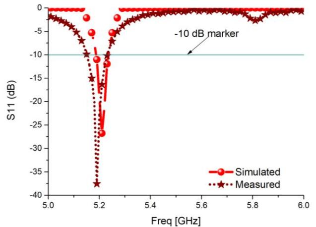
Figure. 7 Simulated and measured S11 parameter
