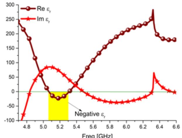
Figure. 5 Dielectric constant of CSRR loaded antenna structure
