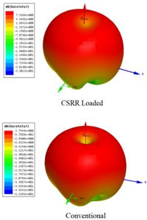
Figure. 9 Simulated gain 3D-polar plot of CSRRs loaded and conventional antenna
