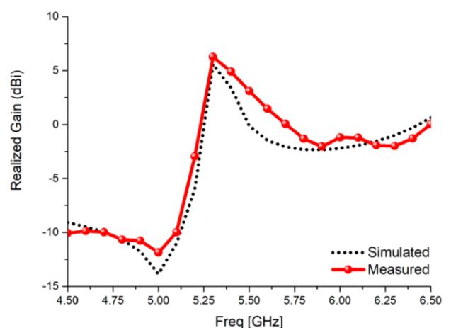
Figure. 8 Simulated and measured realized gain
