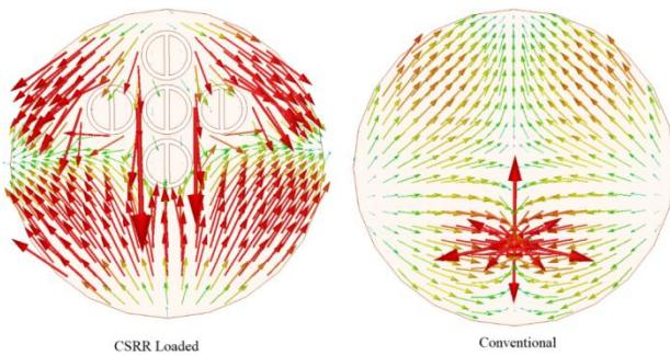
Figure. 2 Surface current distribution on the patch
