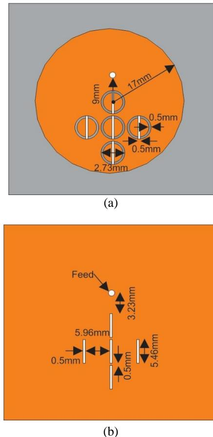
Figure. 1 Configuration of the proposed antenna: (a) top view and (b) bottom view
