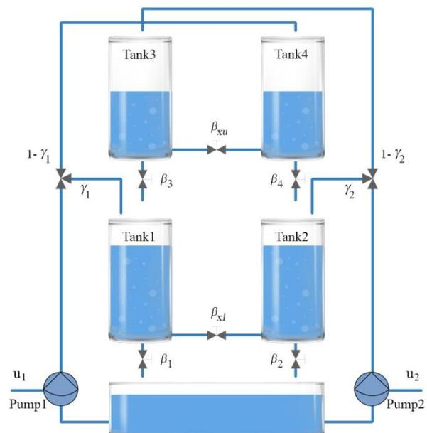
Figure. 1 The multi-configuration tank process: Schematic diagram
