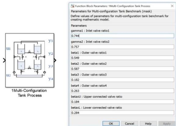
Figure. 4 Block parameters - multi-input multi-output (MIMO) quadruple tank full-interacting process
