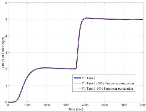
Figure. 14 Step response in case of robustness validation
