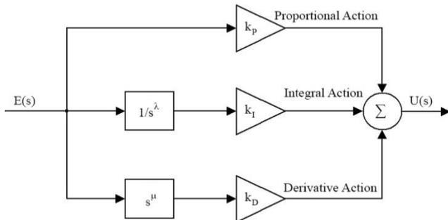
Figure. 8 Block-diagram of the fractional-order  $PI^\lambda D^\mu$  controller
