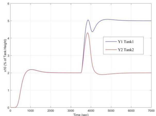
Figure. 12 Step response in case of non-decoupling
