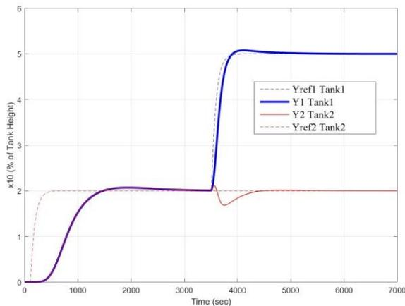
Figure. 11 Step response of multi-configuration tank process simulation: minimum phase
