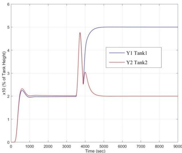
Figure. 16 Step response in case of non-decoupling
