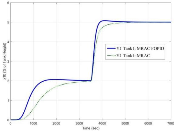
Figure. 13 Step response compared between adaptive fractional order  $PI^\lambda D^\mu$  (MRAC FOPID) control and model reference adaptive control (MRAC)
