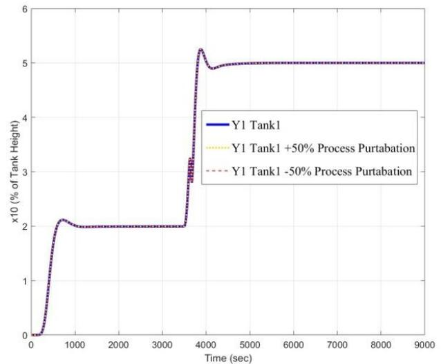
Figure. 18 Step response in case of robustness validation
