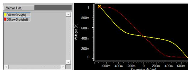
Figure.4 Screenshot of SRAM butterfly curve taken from DC analysis
