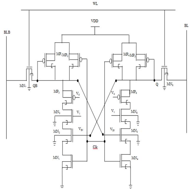
Figure.3 SRAM cell with d-INDEP logic
