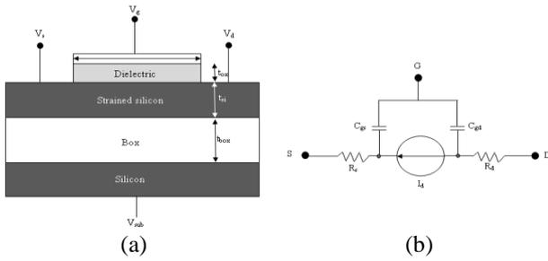
Figure.2 Optimal depleted strained TFET: (a) cross section and (b) equivalent circuit
