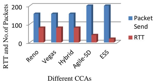
Figure. 8 Packet send ratio for different CCAs with RTT independent ESS
