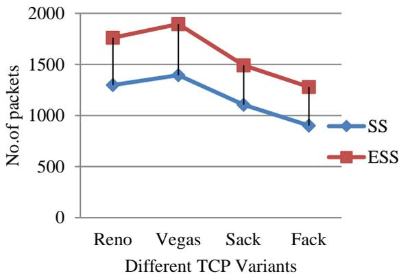
Figure. 5 Packet send ratio for standard slow-start (SS) and enhanced slow-start of different TCP variants
