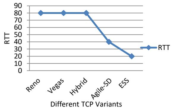
Figure. 7 RTT level for different congestion control algorithms
