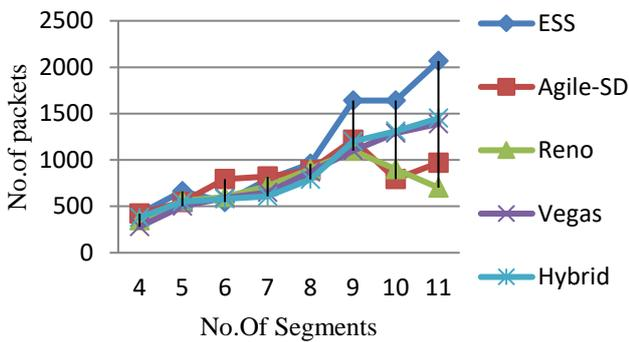
Figure. 4 Packet send ratio for different congestion control algorithm with enhanced slow-start
