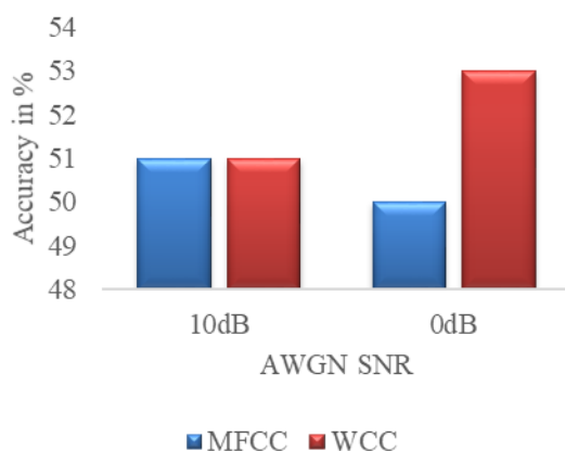
Figure. 8 Detection accuracies of the proposed modified DTW algorithm for half keyword length sequential shift in noisy environment
