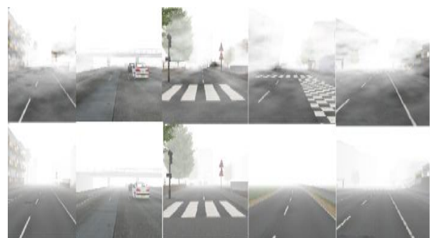
Figure.3 The synthetic hazy images, first row is representing the heterogeneous hazy images, the second row is representing homogeneous hazy images.
