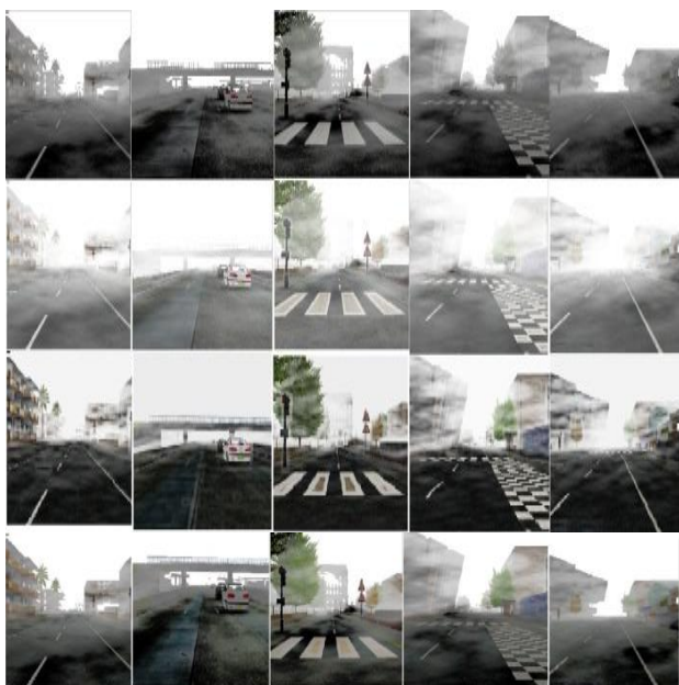
Figure.4 Images of heterogeneous hazy images after applying the algorithms, first row is the proposed algorithms result of first phase, second row is the results of algorithm of Quinsong et al., third row is the result of algorithm of He et al., fourth row is the proposed algorithm result of the final phase.
